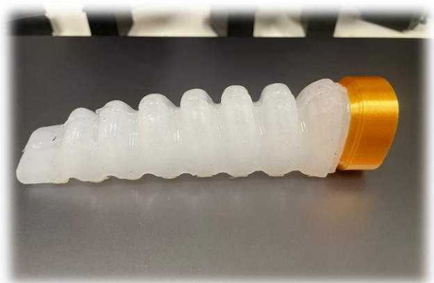
Figure 18. Fabricated Silicone Trilobites Limb
