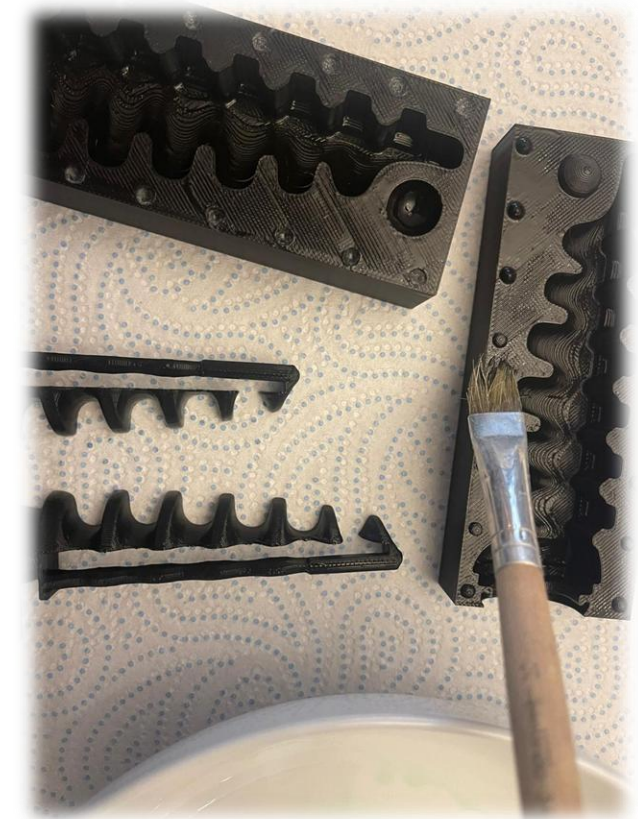
Figure 16. Lubricant Applied to the Mould
