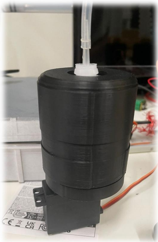
Figure 20. Bellow Actuator Fabricated using 3D printing
