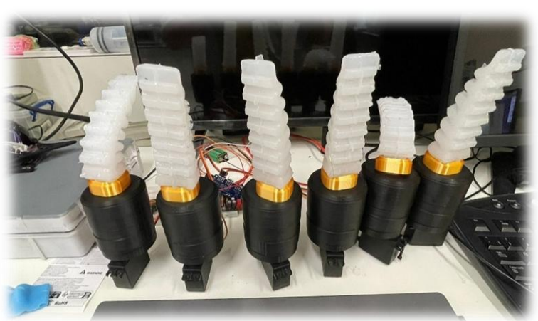
Figure 19. Locomotion Testing of the Limbs with the Actuator
